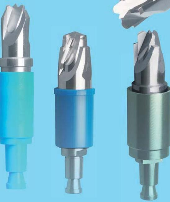
★可超硬、超精研磨，任意的柄部類型、芯厚、容屑槽寬度、刃背方式、鑽尖方式、內冷却孔方式、刃部結構、刃口角度、刃口鋒利程度之要求，及高可至  $\pm 0.003\text{mm}$  ( $3\mu\text{m}$ ) 的尺寸公差要求。We can produce with super hard and super finish grinding and satisfy your requirement of any type of shank, web thickness, width of chip flute, land, drill tip, inner cooling hole, structure of cutting edge, angle of cutting edge, degree of sharpness of cutting edge, and the dimension tolerance can be up to  $\pm 0.003\text{mm}$  ( $3\mu\text{m}$ )
